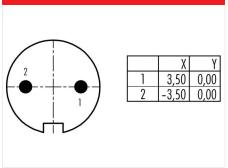
Contact arrangement (Plug-in side)
